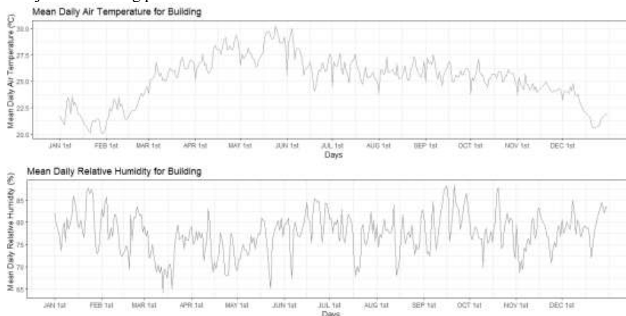
Figure 12. average daily air temperature (Ta) (top) and relative humidity (RH) (bottom) for the entire building over the course of a year
