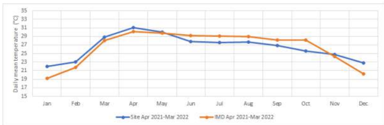
Figure 14. The plot shows IMD temperature data for each month's daily mean temperature, compared with the daily mean temperature by month recorded at the building site using data loggers located in unconditioned spaces throughout the building's corridors.
